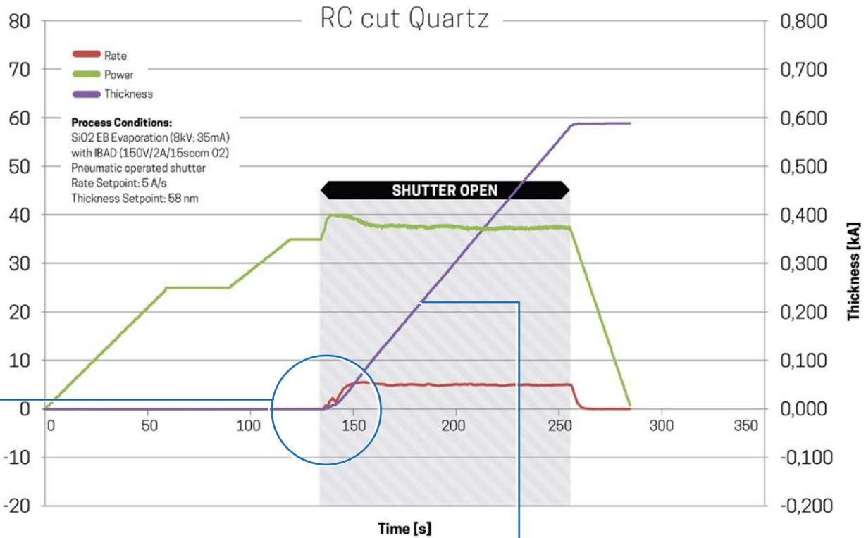
Rate loss prevented by the RC Crystal's mitigation of heat interference
