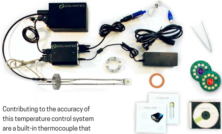
Contributing to the accuracy of this temperature control system are a built-in thermocouple that conveys temperature data to the Eon™ controller - which makes real-time adjustments to the heater - and the Mirage™ air-cooling unit, which automatically delivers super-cooled compressed air into the sensor in response to the fluctuating temperature changes of the sensor.
